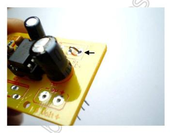
Put the potentiometer in its place. You can only connect this in one way.
