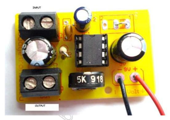
A Budgetronics building kit to make your own mini amp, based on the LM 386 op amp. Handy for amplifying weak signals on a headphone like for instance from a crystal radio. You could also connect a small loudspeaker to it. If you want to amplify a stereo signal you can use two mini amps. One for each channel. Easy connection of output and input signals with block terminals screw connection.
