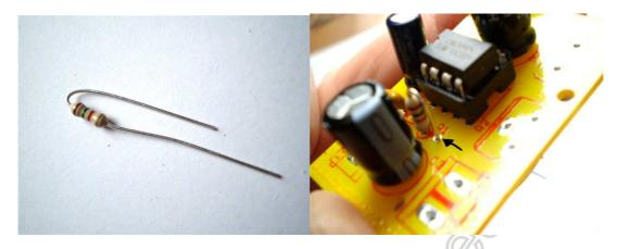
Instead of a switch use a wire bridge. You can use a resistor wire which was cut of in the step before this one. If you want you can install a switch later on.
